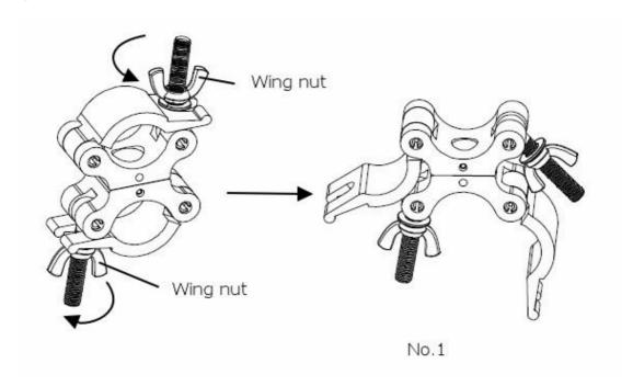
2) Fix the coupler in two pipes, be sure to tighten the wing nuts. Allowing a full 360 degree of movement . Easily fixed in a 90 or 180 degree with a extra pin.(Picture No2,No3)
