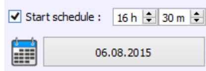
The scene is triggered a single time at the given date and time.
