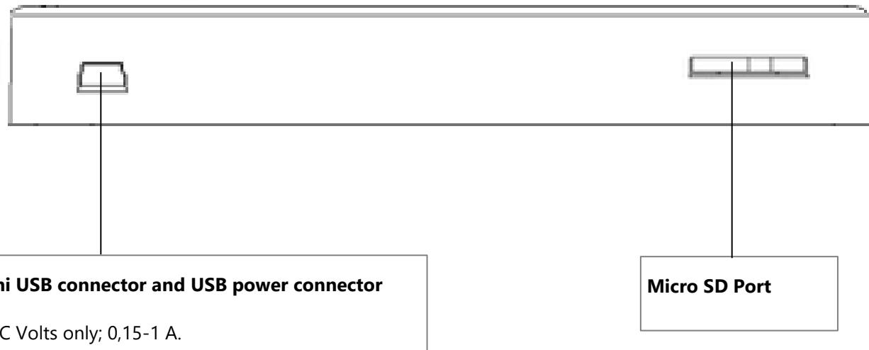
**Mini USB connector and USB power connector**
