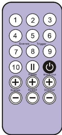
Button 1 to 10 must be assigned to a scene via the software.
