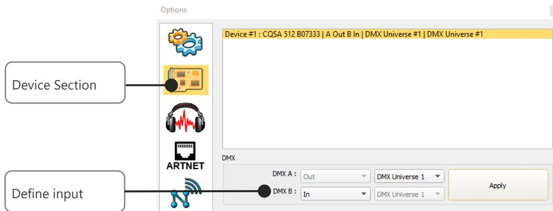
You can select an universe for output and input mode with 1024 and 512 interfaces.
