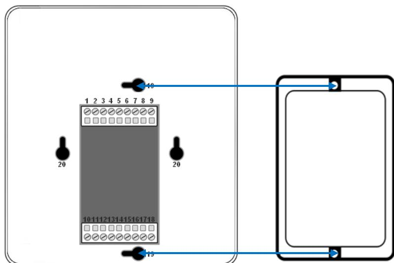
Use the screws of the wall switch box to old the SLIM
